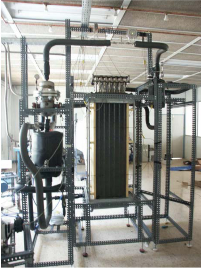
Fig. 5. Falling film absorber experimental test device.
